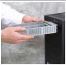
Install Data Express receiving frame into any standard 5.25" bay
