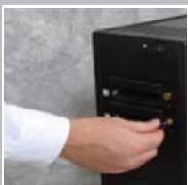
Insert carrier into frame, turn on key lock & press power button
